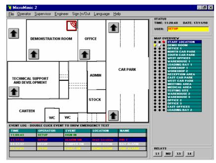
information on which alarms have been triggered. The installer will draw background maps which can link together to cover large buildings or areas. Information on the actions for the operator to perform when a specific alarm triggers is then assigned to each alarm input along with it's priority level, type of alarm and icon design.
